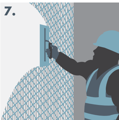
7. Covering mesh with basecoat.
