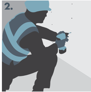
2. Fixing the boards to the background members.
