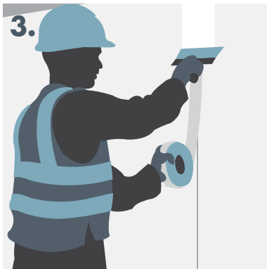
3. Embedding Knauf Aquapanel Exterior Joint Tape.
