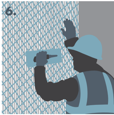
6. Applying reinforcing mesh.
